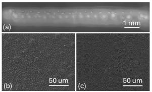
**Fig. 1**. SEM images of AuNP films deposited on a silicon. (a) entire 1 cm deposited line, (b) concentrated nanoparticles in region 1, seen as bright spots on the line, (c) region outside bright spots (region 2).
